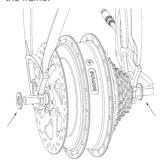
Fasten M12 flange nuts with open spanner at both sides of the motor. (torque requirement: 47-60N.m.)
