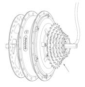
3. Mount a stop pin on both sides of the motor shaft.
