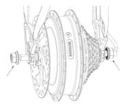
7. Mount the shaft end sheath on both sides of the shaft ends.
