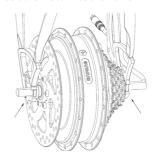
5. Insert a 2mm flat washer on both sides of the frame.
